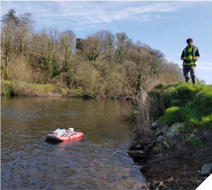
*A remote-control boat: this is used to measure flow and to map the river channel profile.*
