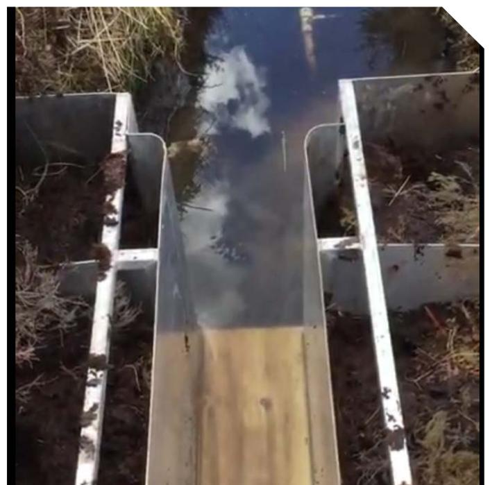
The Living Bog has installed a number of flow measuring structures on selected raised bog project sites. These are used to monitor the discharge and the water quality from the bog. View on YouTube: [www.youtube.com/watch?v=p062FIXesFE](https://www.youtube.com/watch?v=p062FIXesFE)
